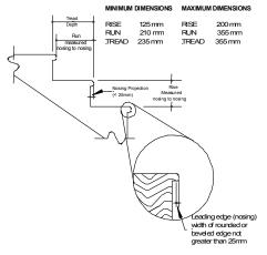
**<u>NOTE</u>**: Exterior wood steps shall not be in direct contact with the ground unless suitably treated with a wood preservative.
